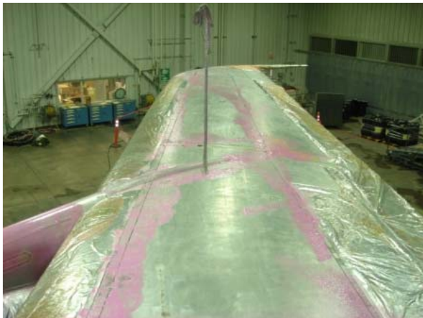
Image 5: Final touch-up strip application of DeKote AF
