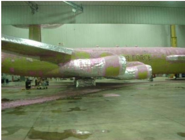
Image 1: First application stripper topcoat & surfacer primer popping off to primer
