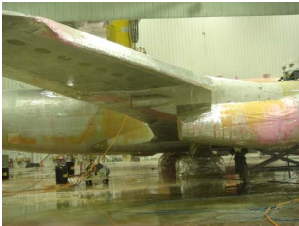
Image 4: Second rinse using power washer with easy removal of primer
